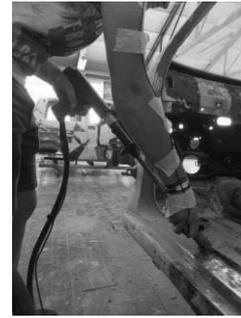
Figure 2. Paintless car dent repair.
