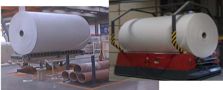
Figure 2 - Raw material loading and transporting (reels)
