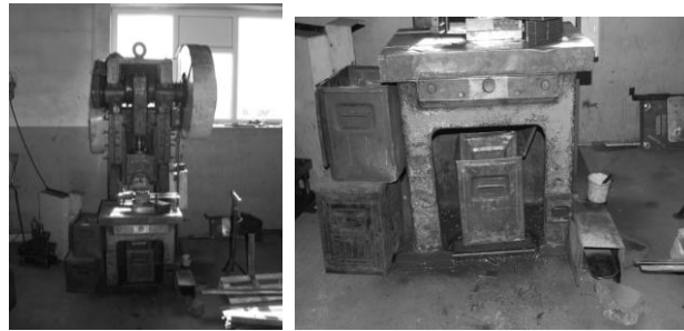
Figure 1 - PMS40B eccentric press and press control system.
