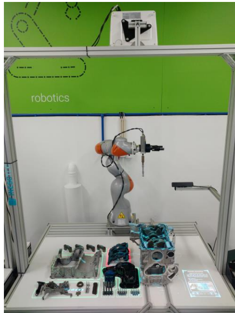
Figure 1. Augmented reality workstation with projected instructions and work zones for the assembly of a car engine.
