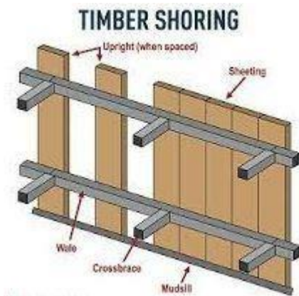
Figure 7. Illustration of timber shoring
