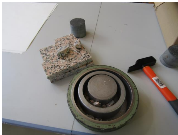
Figure 1. Preparation for grinding granite (2022).
