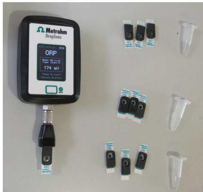
Figure 2. Portable kit for ORP measurements and electrodes (DRP-ORPSEN).
