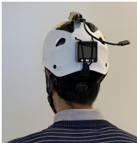
Figure 1. Hardhat system with M5 stack ESP32 integrated as microcontroller.
