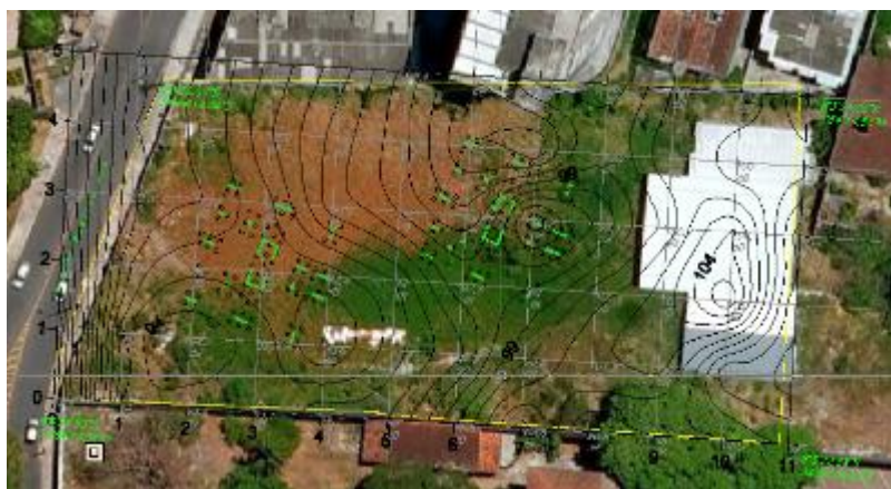
Figure 4 – Map of noise propagation grid points to measure
