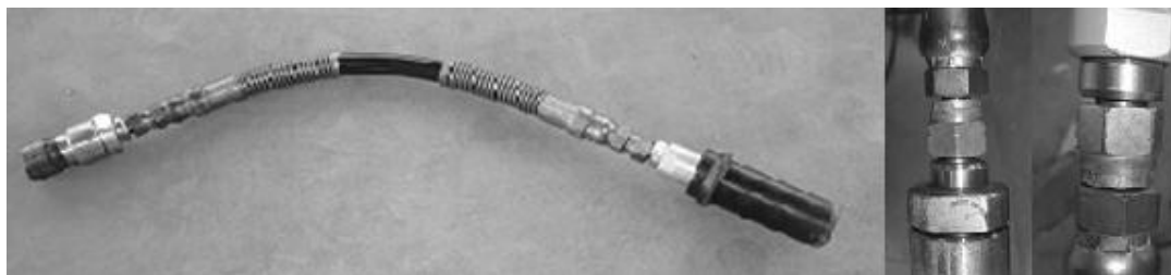
Figure 2 – Reduction coupler (emphasis on union elements)
