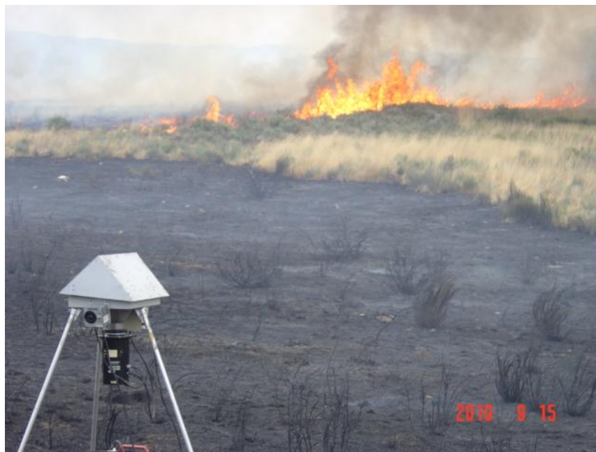
Figure 1. Smoke sampling with a large volume Andersen air sampler.
