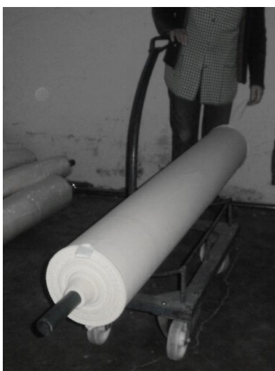
Figure 3 – The load transportation using an improper trolley
