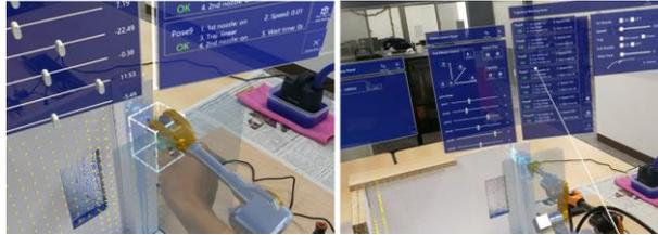
After the planning of the painting task is completed, the self-propelled physical spray-painting robot can move itself to the designated position, which is planned in advance in the virtual environment, as shown in Fig. 12.
