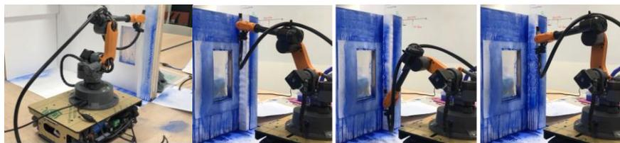
Fig. 13 The physical spray-painting robot performing painting tasks
