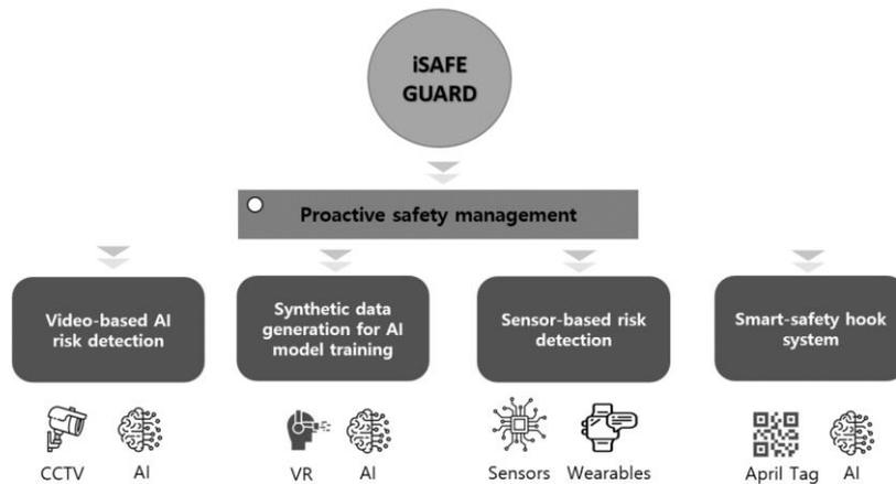
Fig. 6: iSAFEGuard's technological functionality.
