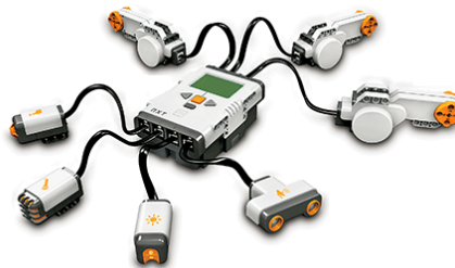
Fig. 1. Lego NXT brick and some of its sensors and servo-motors.
