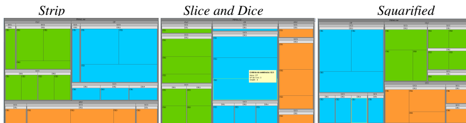
Fig. 9. Treemaps for data structure of Table 2, with different division algorithms.
