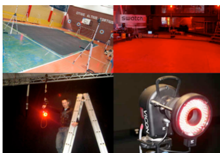
Figure 3: Upper left: A mocap studio. Upper right: Same mocap studio during capture. Lower left: A motion capture camera. Lower right: Close-up of a motion capture camera.
