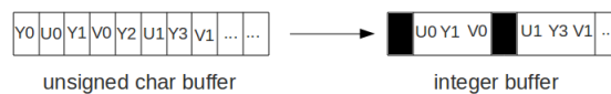
Fig. 5: An illustration of the conversion of the unsigned char buffer to an integer one, allowing thus the reading of 4 bytes at the same time. Using this approach we can obtain a reduced resolution of the images.
