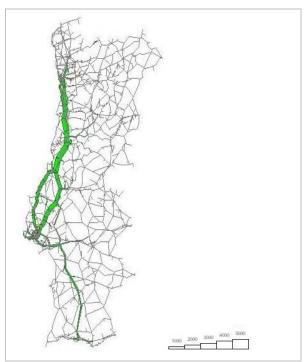
**Figure 8.** Change on road traffic flows resulting from HSR introduction (Week Am Peak) – Green represents the traffic reduction and red the traffic increase
