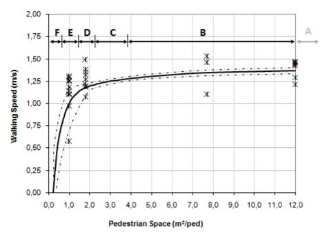
Figure 2. Walking speed at Cais do Sodré Station
