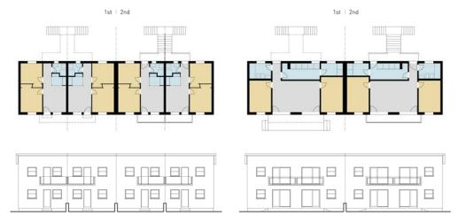
Figure 2. Left: set of four original Type2 (8xT2) houses. Right: renovation proposal typology (4xT2)
