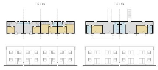
Figure 6. Left: set of four original Type4 (4xT3) houses. Right: renovation proposal typology (4xT1)
