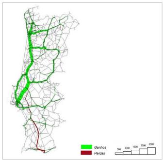
**Figure 10.** Change of passengers flows on bus network, resulting from introduction of new headways calculated in Regulatory Scenario (morning peak period)
