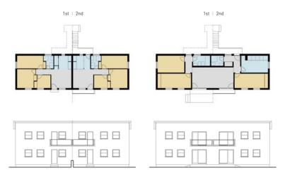
Figure 4. Left: set of two original Type3 (4xT3) houses. Right: renovation proposal typology (2xT3)
