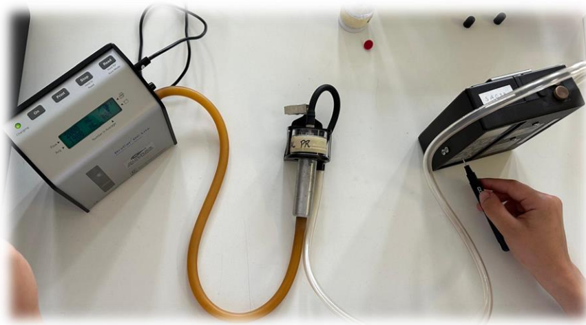
Figure 2: Pumps calibration/verification process.
