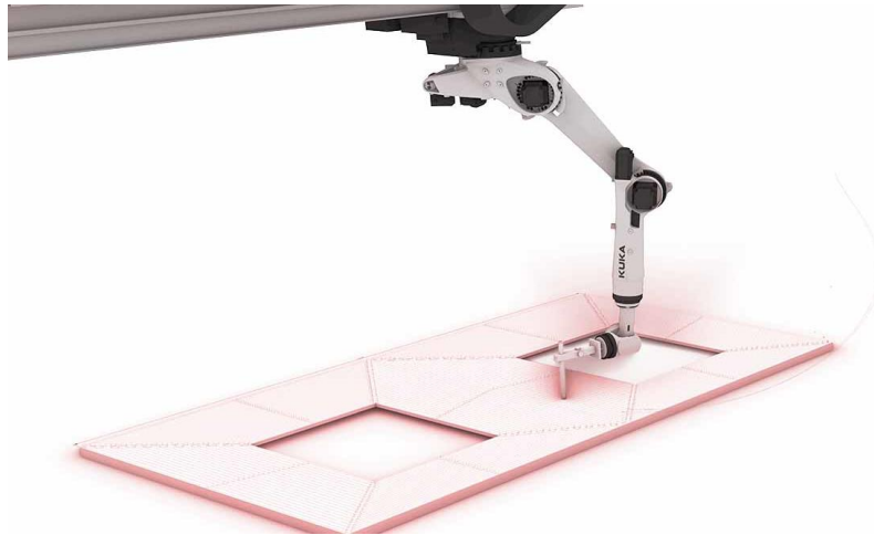
Figure 5: Robotic toolpath generated from the parametric façade geometry, illustrating the continuous extrusion strategy adopted for 3DCP.
