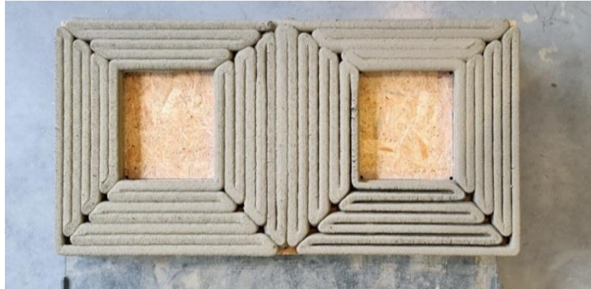
Figure 6: Scaled 3DCP prototype produced to preliminarily validate the proposed BIM-driven RF workflow.
